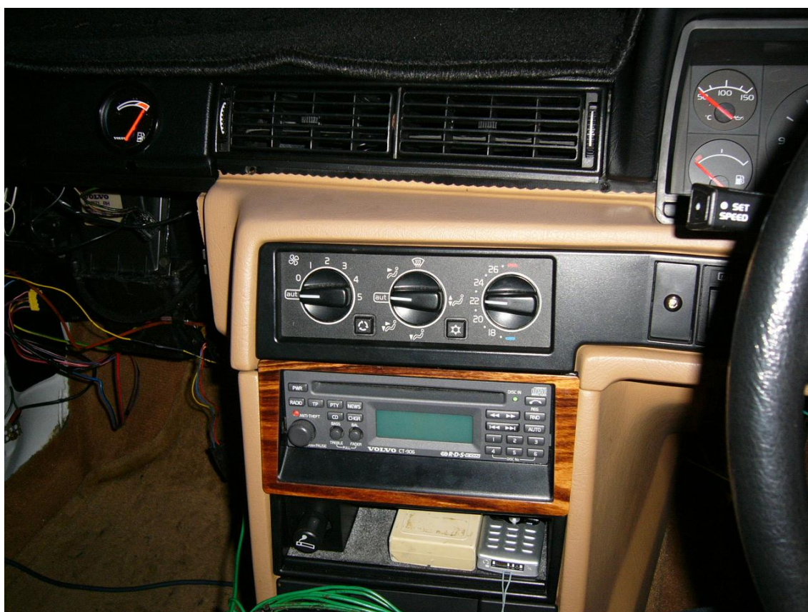
Above : My dash re-installed, as well as the ECC control panel.
